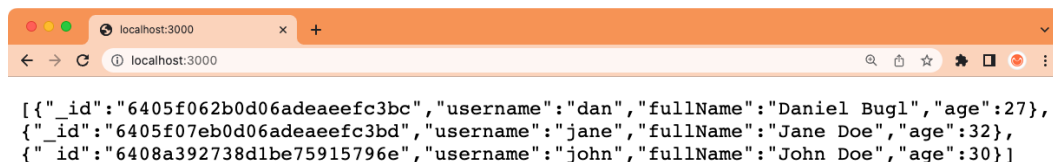
Figure 2.14 – Our first Node.js service retrieving data from a MongoDB database!
